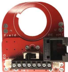
Figure 3 Field Panel Printed Circuit Board Part: RS32F
