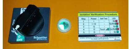
SwitChek is a 3 phase, Isolation Switch Tester. As a switch resistance tester it confirms that an isolation switch or circuit breaker does not pass electrical voltage or current when isolated.
